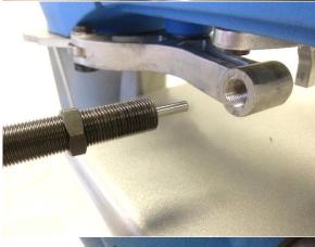
Unthread old Shock Absorber from Rocker Arm using 5/16" Combination Wrench
