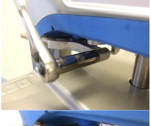
Loosen Retaining Nut on old Shock Absorber using 9/16" Deep Well Socket or Wrench
