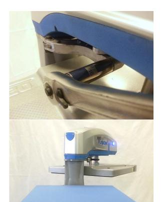
Tighten Retaining Nut using 9/16" Deep Well Socket or Wrench
