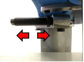
If Heater and Lower Platen are not aligned, adjust Shock Absorber by threading in or out
