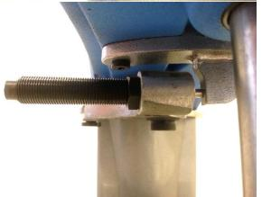
Thread new Shock Absorber onto Rocker Arm, up to Retaining Nut (hand tight)
